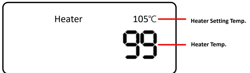
Figure 9. Main Display shows heater temperature during running
