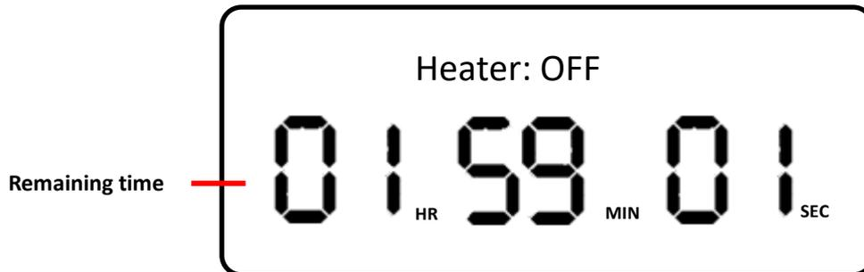
Figure 8. Main Display shows countdown time during running
