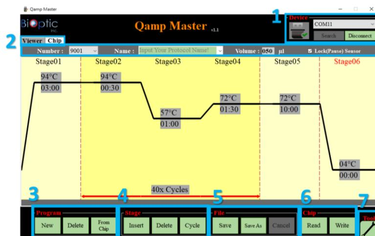
Figure 12. The main interface of Qamp<sub>mini</sub><sup>TM</sup> Master after reading the Programmable Chip
