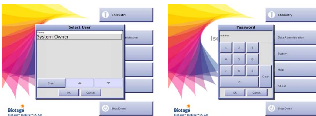
Figure 2-1. Log into the Data Administration Mode (Isolera LS with Spektra License Shown)
