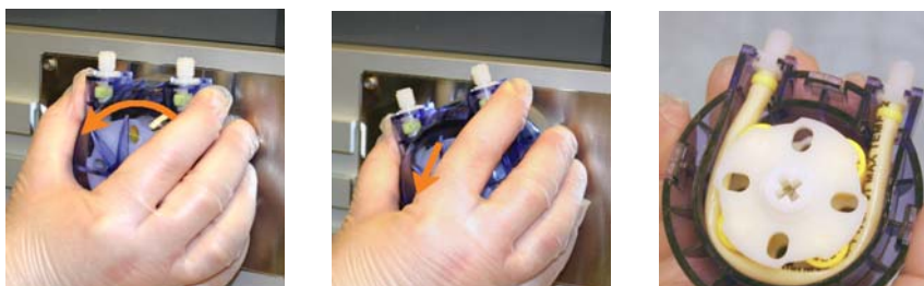
Figure 4-12. Remove the Sample Loading Pump
