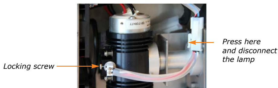
Figure 5-15. Disconnect the Tungsten Lamp
