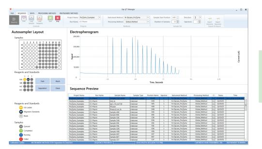
Figure 3: Gly-Q Manager Sequence Tab. Sample set-up and real-time data acquisition window. Samples are loaded in a 96-well plate, reagents for instrument functions and required standards are loaded in a dedicated instrument tray. Real time data and system progress by sample are displayed.
