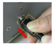
Pull the connector header to unlock and detach the cable from instrument
