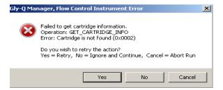
**A.** Insure that the cartridge is installed correctly as per section 3.6.2, above.
